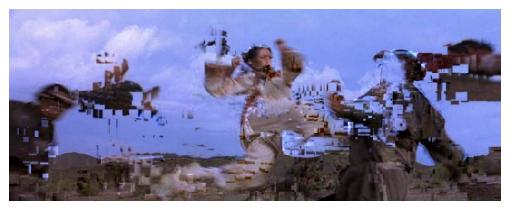
Figure 5: Mpeg4, Drop = 0.1%, Delay = 1.5 ms and Jitter = 0.025 ms
