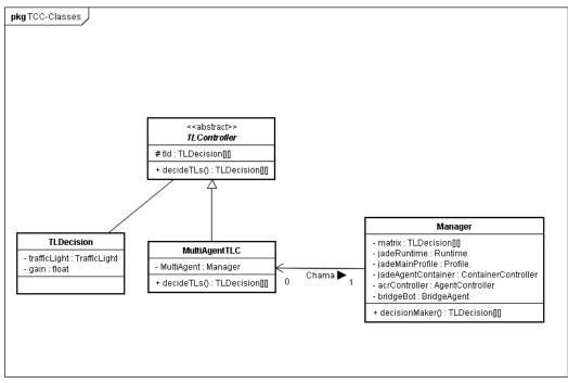
Figura 4: MAS connection to GLD through TLController
