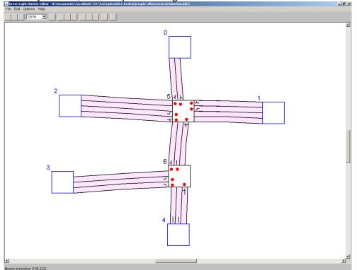
Figure 5: The blue nodes are entry and/or nodes and the black ones are intersection nodes, the red dots are traffic lights
